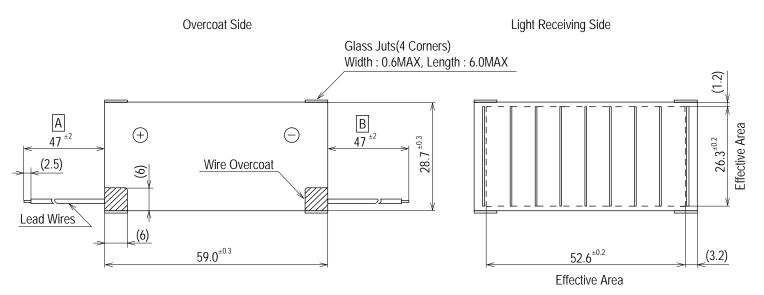
Note: Glass Substrate Thickness : 1.1mm Module Thickness : 1.3mm max
